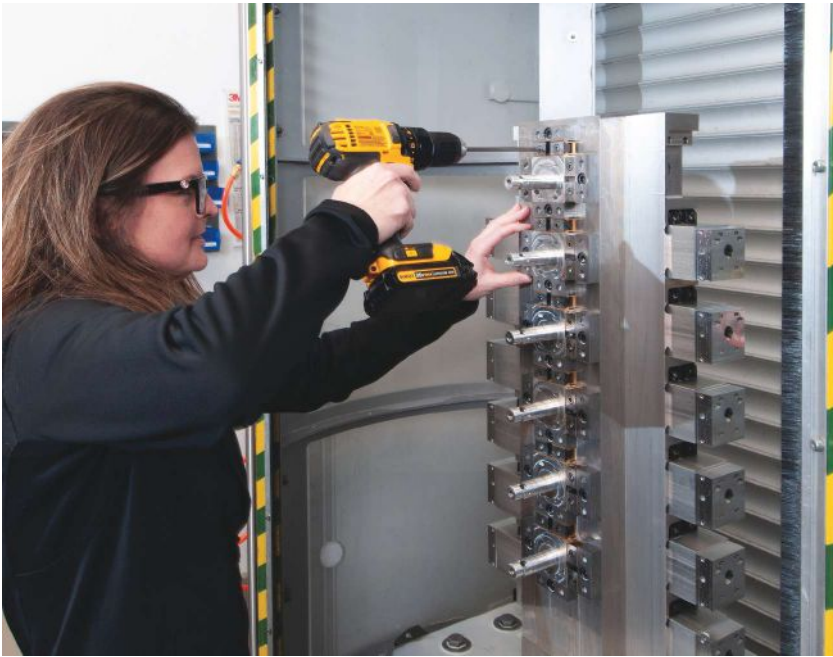
Mach Machine operations manager Angela Olsen secures a workpiece onto a pallet in the shop's Fastems FMS One flexible manufacturing system. Moving to permanently setup tombstones like this has greatly improved efficiency and productivity for the burgeoning machine shop.
