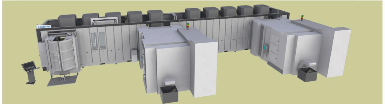
*Mach Machine, Inc. recently expanded its automated production capabilities with the addition of two Okuma MB5000H attached to a 24-station Flexible Manufacturing System (FMS). This is a lights-out manufacturing system that operates unattended, day and night.*
